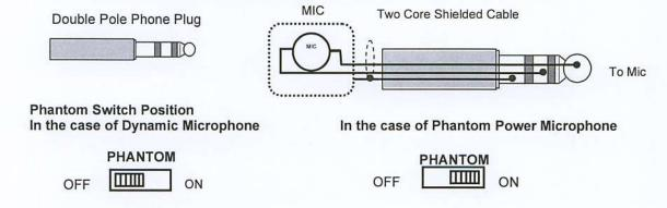
However, the microphone input circuit is in a condition of unbalance when it uses Single pole type. Because it is easy to pick up noise with the state of unbalance, the length of the microphone cable recommends what is used at less than 10m.
