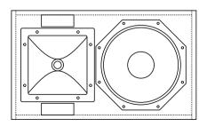
rotate HF horn 90° for horizontal orientation
