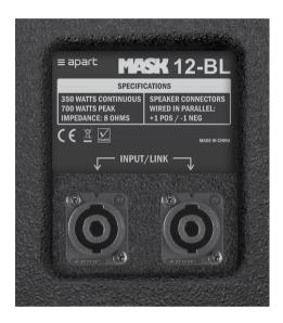
Input: the signal from a power amplifier must be connected to the input/link speakon® connector. The connectors are equivalent and internally wired in parallel. Connector 1+ (positive) and 1- (negative) are used. 2+ and 2- are not connected.
